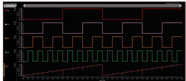
Fig. 6. Characteristic curves of the  $16 \times 1$  multiplexer from software Virtuoso Cadence®.
