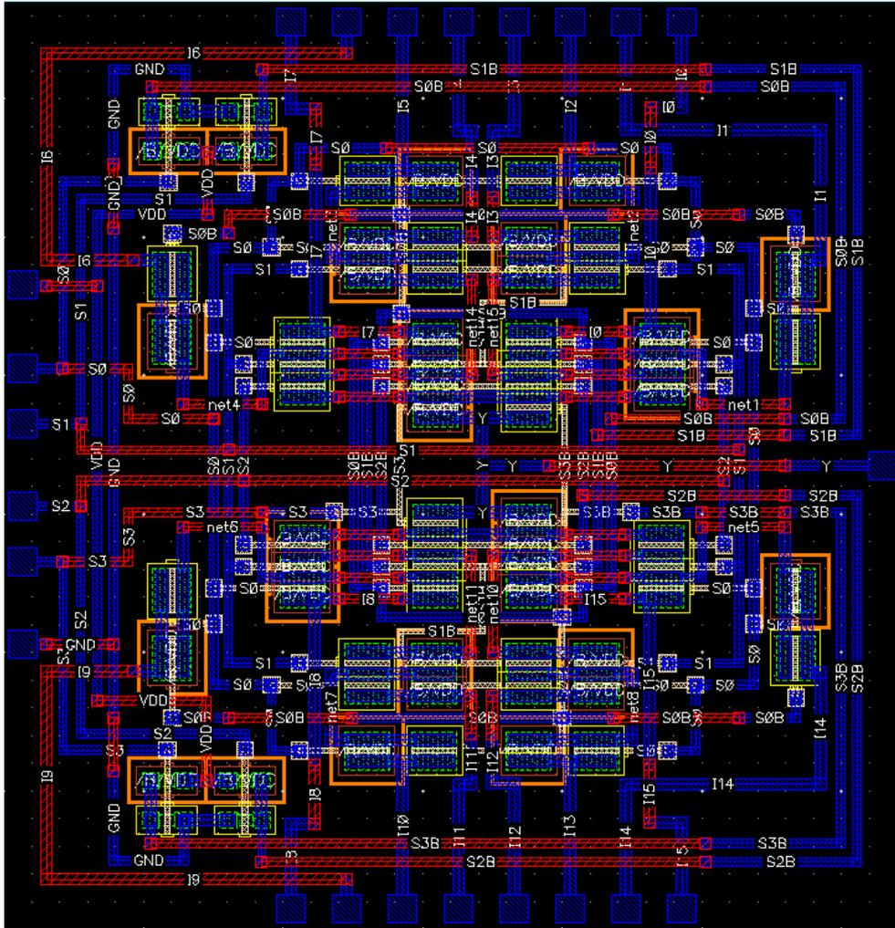
Fig. 7. Fabrication layout of the 16 x 1 multiplexer from software Virtuoso Cadence®.
