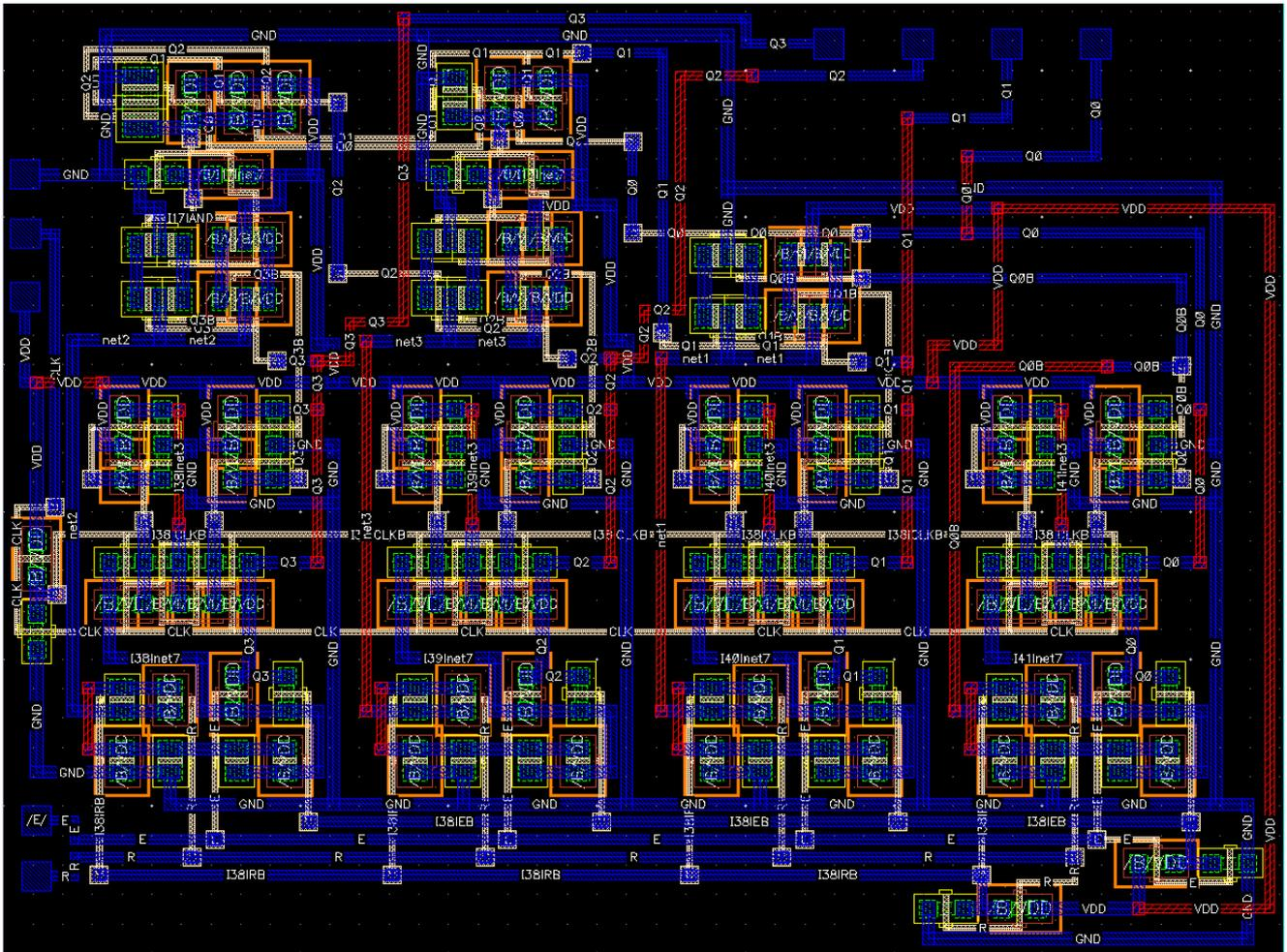
Fig. 4. Fabrication layout of the 4-bit counter from software Virtuoso Cadence®.
