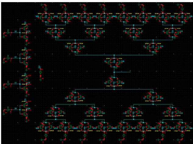
Fig. 5. Schematic of  $16 \times 1$  multiplexer from software Virtuoso Cadence®.
