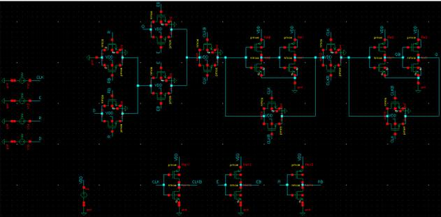
Fig. 1. Schematic of Flip-flop D from software Virtuoso Cadence®.
